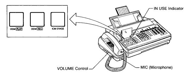
Make sure that the micro cassette tape is properly installed. (See page 1-8.) The recording time is limited to 16 seconds.
